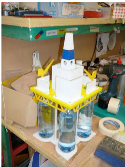
The Oil Rig Model showing lemonade bottles, and holes in superstructure for air to escape.
